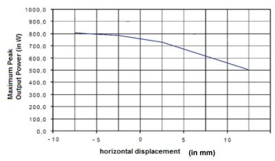
Fig. 1: Output power on aluminum track, e.g. EMS
